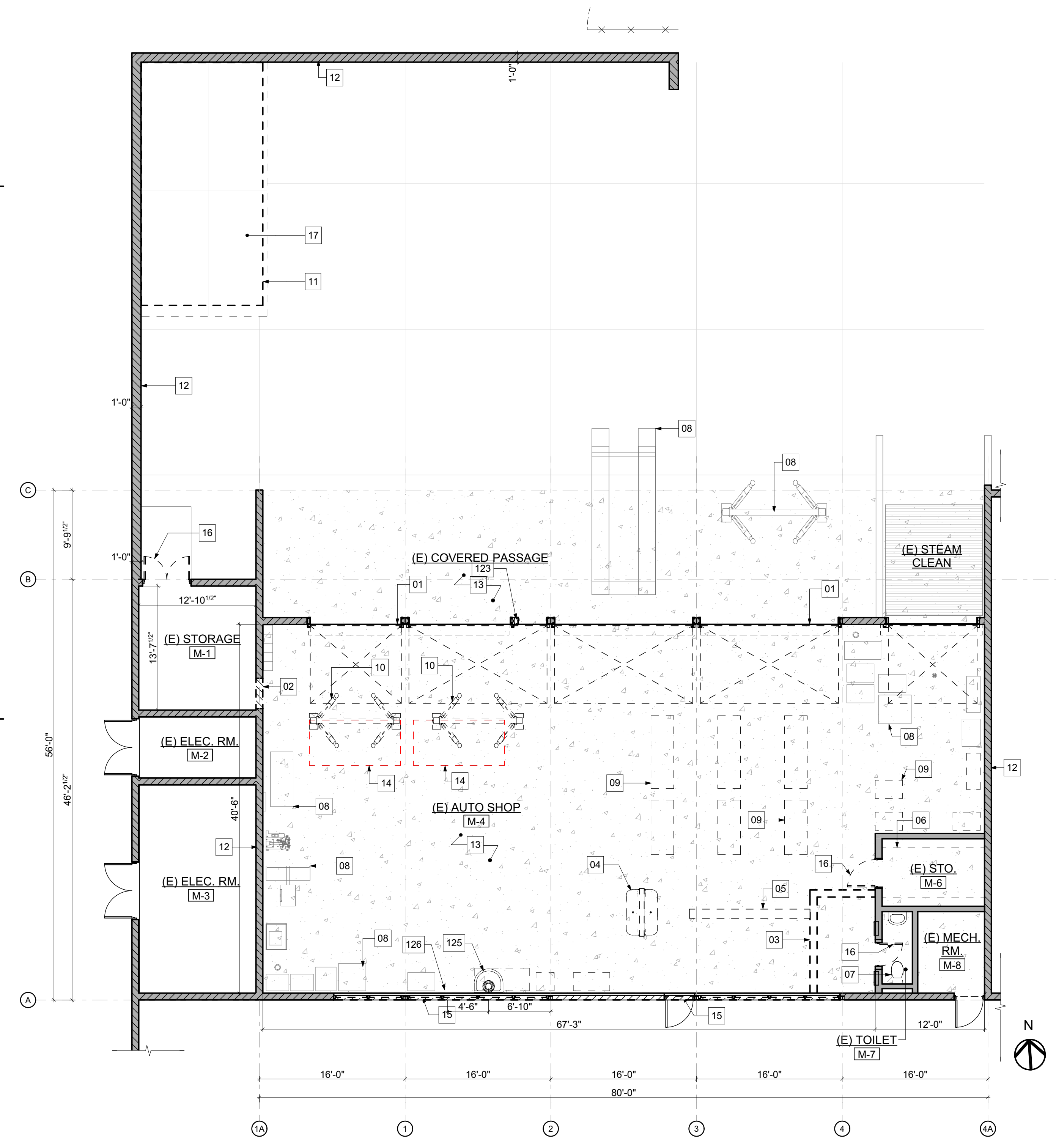
DEMOLITION FLOOR PLAN 2 SCALE: 1/8" = 1'-0"
